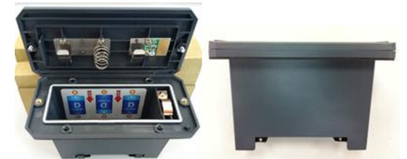
Figure 3 The correct orientation of the cover of the cell box.
