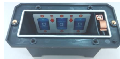
Figure 1 Polarities of batteries.
