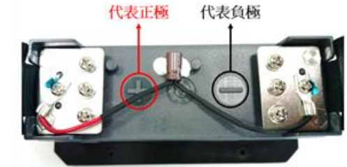
Figure 12 Wiring Diagram of the cell box
