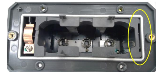
Figure 4 The right direction of the cell box holder.
