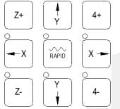
• Control the axis movements, able to fast travel when pressing the rapid button with arrow keys at the same time.
